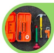
**Operation and maintenance kit:** A WASH operation and maintenance kit should include 1 screwdriver, 1 toilet plunger, 1 hammer, 2 pipe wrenches, 2 extra faucets, spare paint (**total cost around M2100**)
